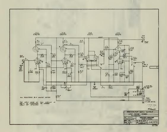
Fig. 12. Low-noise-model preamplifier (125 Ωoutput).
